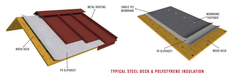
Renderings provided for general assembly clarification. Atlas recommends that installed slipsheet roll direction have a perpendicular relationship to installed membrane roll direction.
